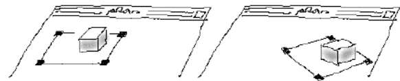
Figure 3. Move and rotate virtual object by manipulating a physical brick, which acts as a handle.
