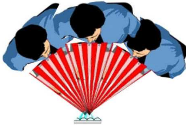
Figure 2. Three viewing zones consisting of nine different perspective views each. The repetition of viewing zones enables multiple viewing.
